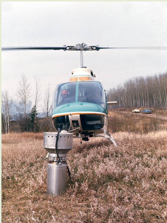
Original "ping-pong ball" aerial ignition device built by the Alberta Forest Service's Roy Kruger from an Australian prototype developed at the Northern Forestry Centre; late 1970s
